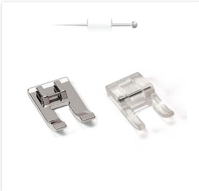
The Open Toe Foot can be used for machine applique, decorative stitching and many types of surface embellishment. The foot provides a clear view of the stitching area, and the tunnel on the underside of the foot allows dense stitches or raised trims to feed smoothly under the foot.
