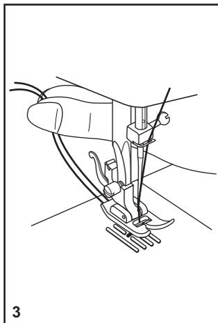
Gently pull on the upper thread to bring the bobbin thread up through the needle plate hole (2).
