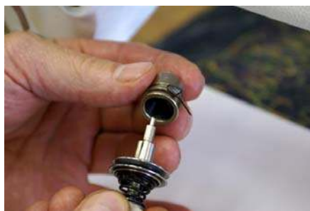
Fig 17: Insert the tension assembly back in barrel
