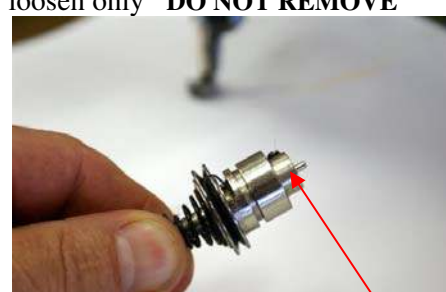
Fig 6: Tension assembly out of machine DO NOT LOOSE PIN
