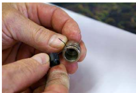
Fig 14: Insert New Spring
