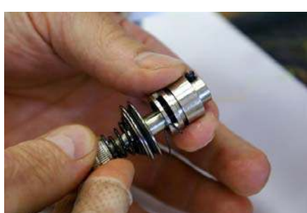
Fig 8: Remove tension assembly from barrel
