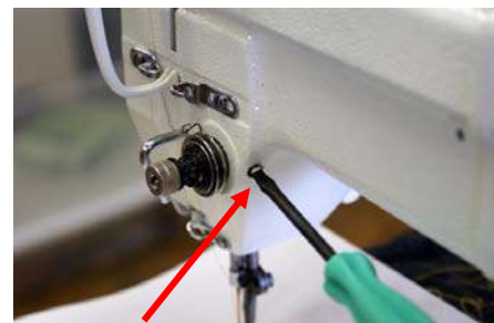
Fig 3: Screw on inside of machine loosen only DO NOT REMOVE
