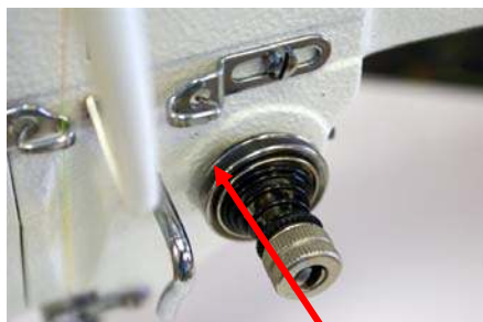
Fig 1: Tension Assembly with broken Spring (old tension knob)
