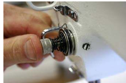
Fig 24: Release and the disk will close; this is the proper place for your tension assembly
