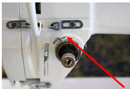
Fig 26: Tension assembly back in place with new check spring at 11:00
