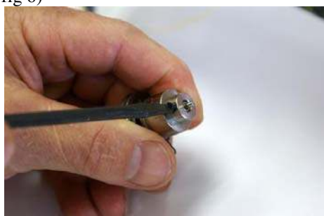
Fig 7: Loosen screw only DO NOT REMOVE
