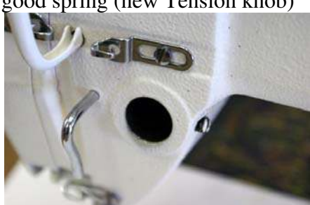
Fig 5: Machine with tension assembly removed
