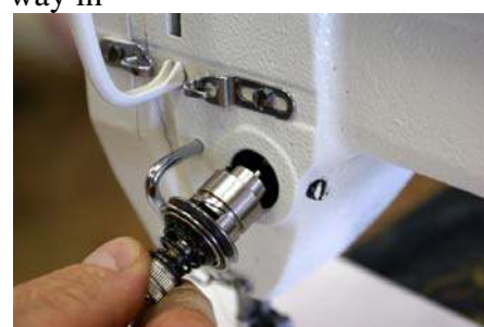
Fig 21: Place the assembly back into your machine
