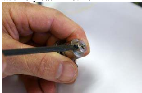
Fig 20: Tighten screw. Make sure pin is still there
