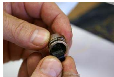
Fig 15: Twist while inserting new spring
