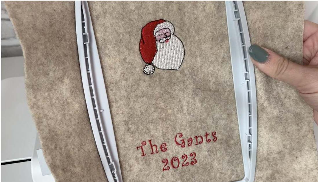
21. Loosen the screw on the hoop and separate the inner and outer hoop pieces to release the fabric and stabilizer.
