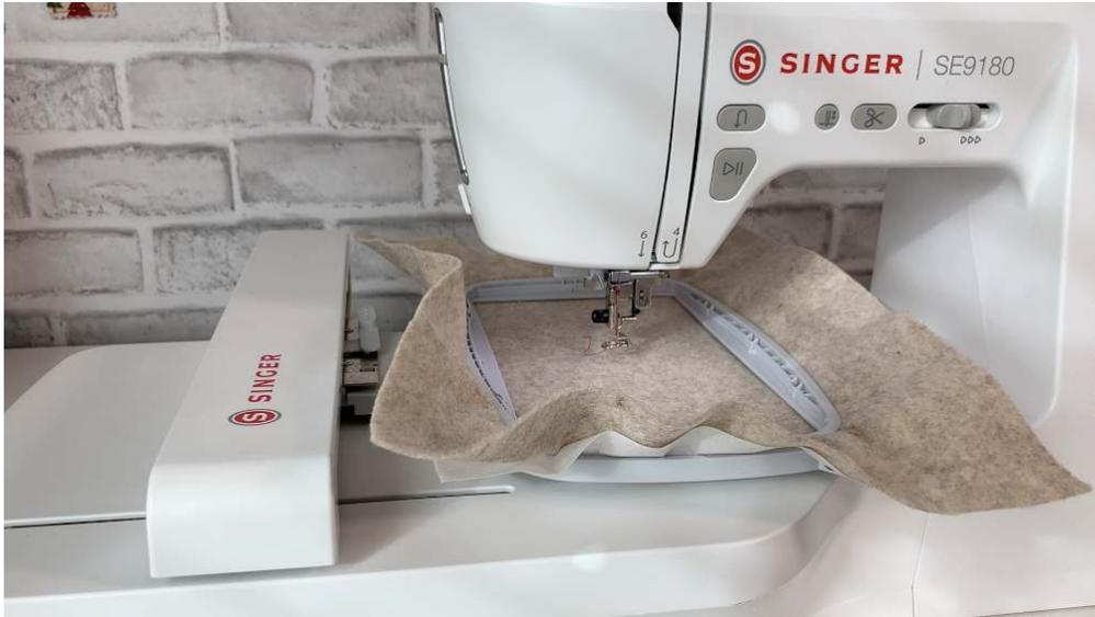
17. Thread the machine with the first rayon thread color for the design. Lower the embroidery foot.
